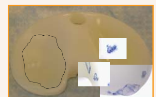
Figure 4: Methylene blue allows edge impingement, pitting, and delamination to be recorded for each poly insert. The wear scar is outlined with the black line for analysis of area for each insert as well.
