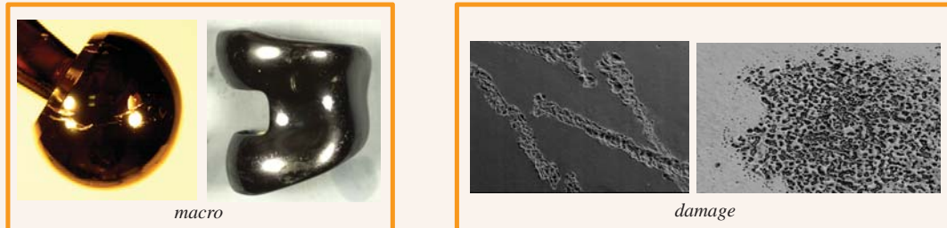
Surface damage from instrumentation: altered polyethylene wear phenomena
